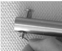
remove stopper pin, cottor pin and washer
