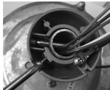
reinstall half-ball with stopper pin and tighten set screw
