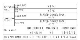
NOTEI. CUT THE DRAIN HOSE (ACCESSORY) FOR USE, IF NECESSARY.
