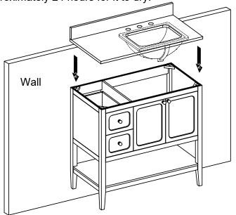
Step 6 Notes: Apply silicone caulk (not included) to unpolished side and bottom of backsplash. Position backsplash on top and against wall. Clean any excess caulk beforeallowing to dry.  $\checkmark$
