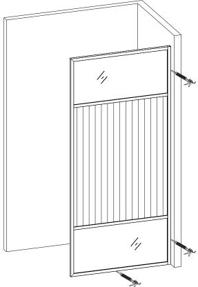
Please ensure the bottom horizontal is straight before the silicone sealant to cure fully
