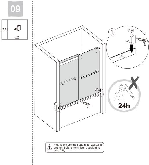
• Do not use the shower enclosure for at least 24 hour in order to allow the silicone sealant to cure fully.
