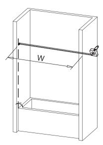
2. Your Upper Guide Rail [5] and Bottom Guide Rail [9] have been precut for your Shower model opening width, eg.60" for shower width. If W-width of your wall-to-wall opening is equal to the size of your Shower model, it is unnecessary to cut the Upper Guide Rail and Bottom Guide Rail and you can continue to Step 3.
