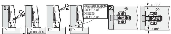
1. Adjusting screws on the hinge arm can adjust the front and rear of the door panel
