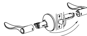
Note: Levers can only be removed when the lock is unlocked
