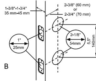
Common Standard for Lock Height off Floor is 36" to 39" above the floor.
