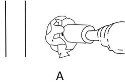
B) Drill the 1" Latch Hole from the door edge fully into the Lock Bore hole
