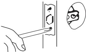
Install Latch in the up position as marked on the latch.
