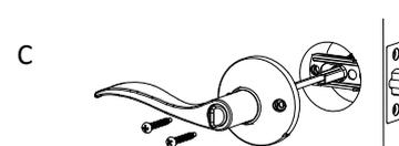
Note: Check alignment of the lock as you tighten the screws to keep lock centered over the bore Hole
