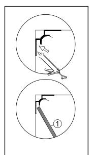
6. Press against the wall smoothing out any air bubbles along the entire area and then lightly tap on wall panel with a rubber mallet from top to bottom to ensure it is tightly connected to the wall.
