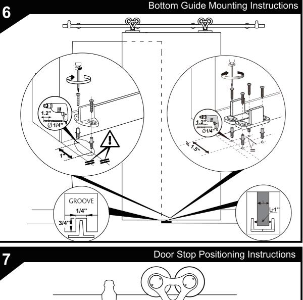
The Guide Stabilizes the door by keeping the bottom from Swinging. Kit includes both a Mortise (Grove in the bottom of the door) and a Non-Mortise option.
