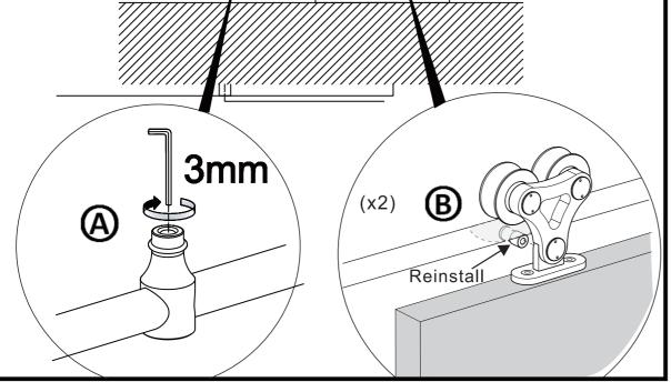
B Reinstall Auti-jump pins to keep door safely on the rail when in use
