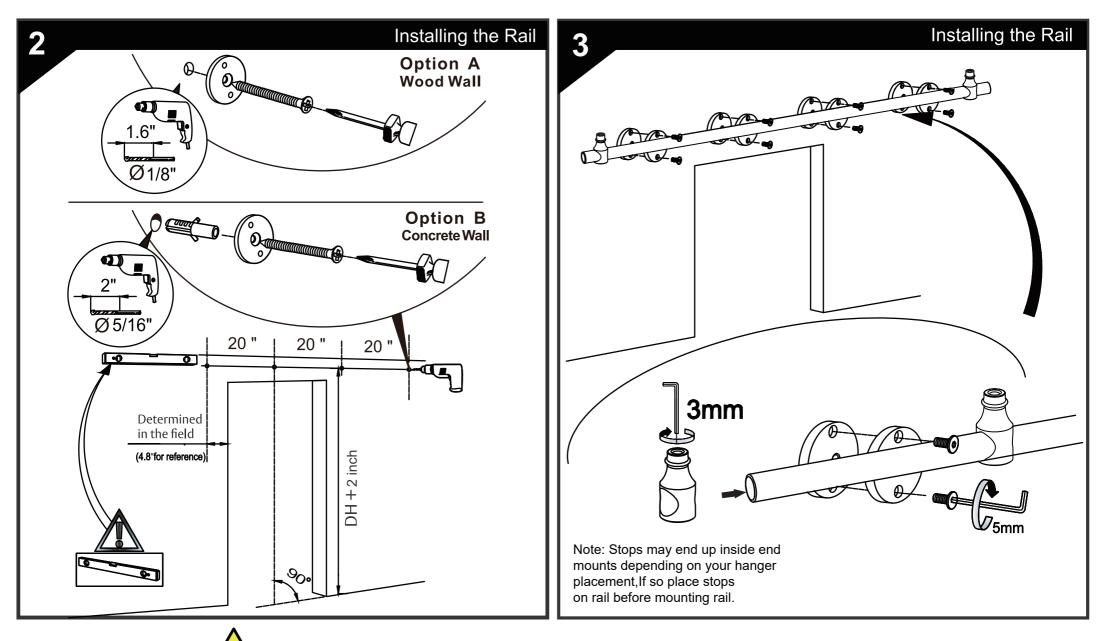
All Rail Mounts must be screwed into a solid Wood Header
