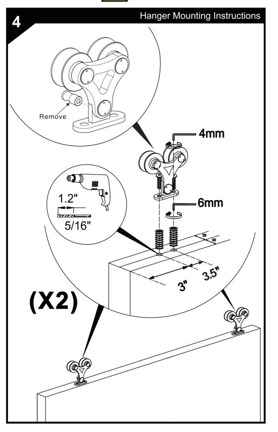
Hanger position from the edge can vary based on your door design. Position Shown is for a flat Surface Door you may have to Adjust to center Hanger onto the vertical styles of your door
