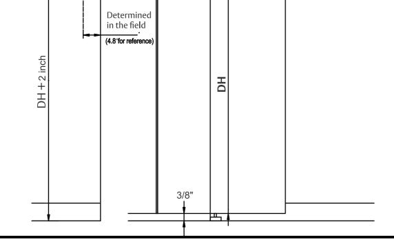
Recommend that you layout your door and hardware on the floor first to determine spacing.
