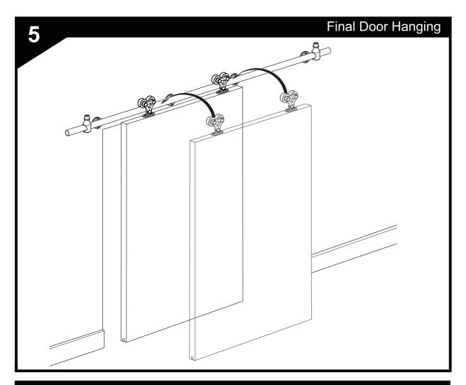
Hang the door and slide it into the Floor Guide .
