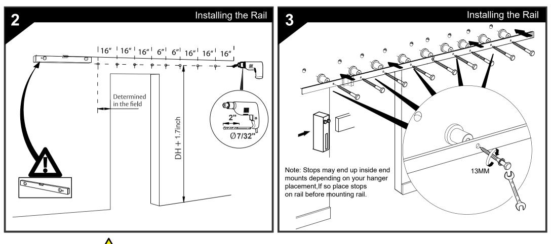
All Rail Mounts must be screwed into a solid Wood Header
