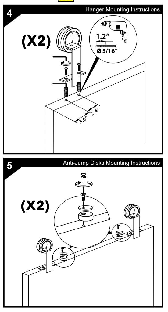
Hanger position from the edge can vary based on your door design. Position Shown is for a flat Surface Door you may have to Adjust to center Hanger onto the vertical styles of your door
