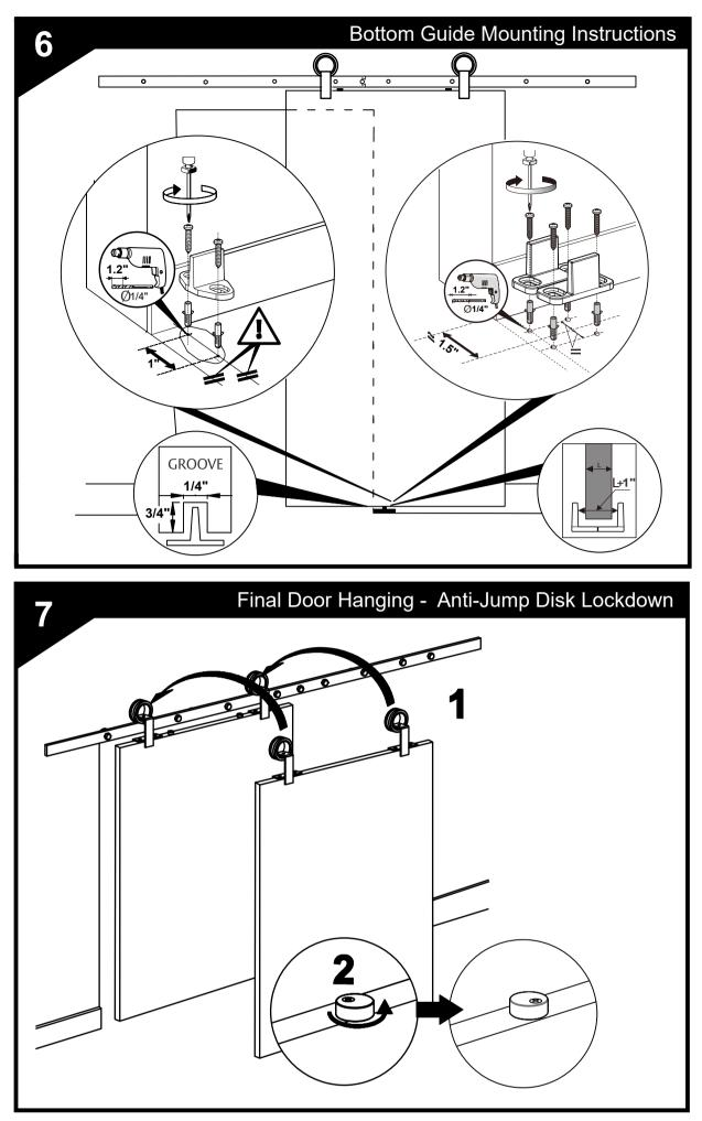
The Guide Stabilizes the door by keeping the bottom from Swinging. Kit includes both a Mortise (Grove in the bottom of the door) and a Non-Mortise option.
