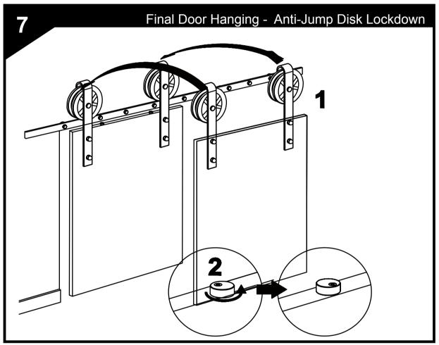
Hang the door and slide it into the Floor Guide then Rotate the Anti Jump Disks under the rail and tighten down the screws to lock them in place
