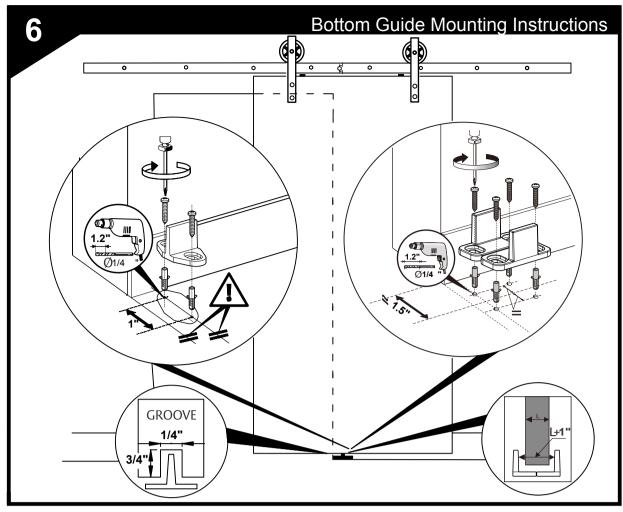
The Guide Stabilizes the door by keeping the bottom from Swinging. Kit includes both a Mortise (Grove in the bottom of the door) and a Non-Mortise option.
