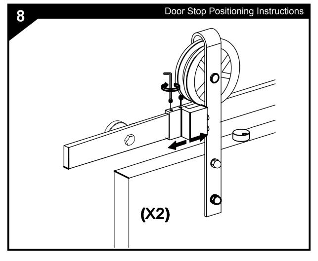
Adjust your Door Stops to your desired position and lock down your Door Stops with the Allen Wrench Provided
