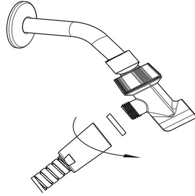
Hand-tighten the other end of the hose onto the water inlet.
