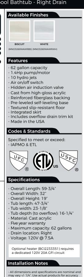
in critical situations.Tub must be supported from the tub bottom and not the tub lip or stringers. Failure to do so will void
