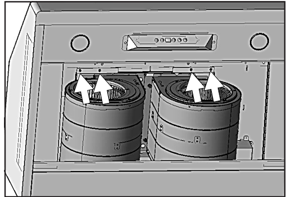
2. Remove (4) screws attaching dual blower plate to top of interior body of hood. Remove dual blower from hood body.
