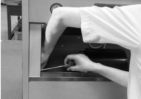
1. Unscrew (2) screws holding each left and right side bottom spacer panels and remove panels from hood body.
