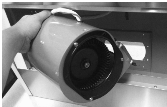
6. Remove blower from hood body and turn blower 180 degrees so that blower outlet faces the back of hood body.
