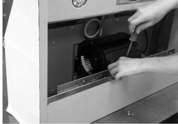
2. Unscrew (4) screws holding the rear filter holder panel and remove panel from hood body.
