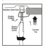
7.Rotate the clamp on the clip 90 degrees to the channel and tighten screw clockwise. from the center clip using a long screwdriver.
