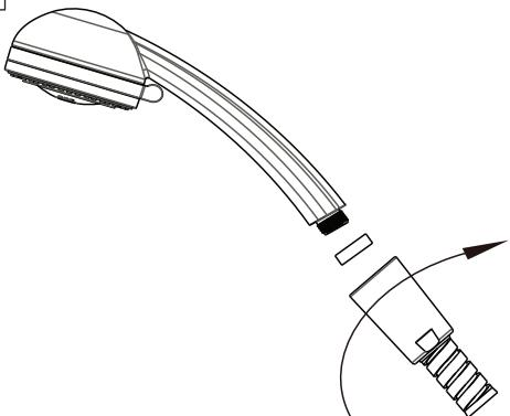
Place washer into end of hose and hand-tighten hose to the bottom of hand shower.
