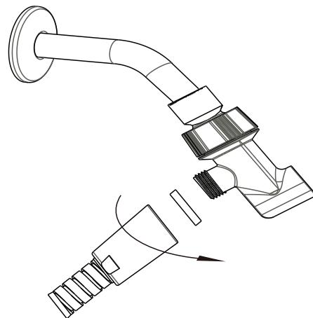
Hand-tighten the other end of the hose onto mounting bracket or 3-way diverter.
