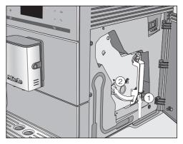
Press and hold the button under the brew unit handle ① and, while doing so, turn the handle to the left ②.
