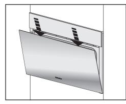
Using two hands placed on the upper edge of the door, push the door downward briefly.
