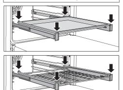
The FlexiClip telescopic runners can support a maximum load of 33 lb (15 kg).
