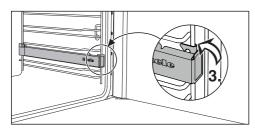
Then secure the FlexiClip telescopic runner to the lower rail of the shelf level (3.).
