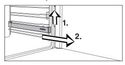
■ Remove the FlexiClip telescopic runner by raising it at the front (1.) and then pulling it forward along the rail of the shelf level and out (2.).
