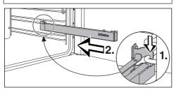
■ Hook the FlexiClip telescopic runner onto the lower rail of a shelf level at the front (1.) and push it along the rail into the oven compartment (2.).
