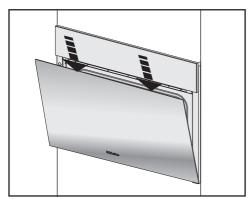
Using two hands placed on the upper edge of the door, push the door downward briefly.
