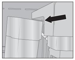
Attach the milk valve cover as follows: insert the pin in the top righthand corner and swivel the cover backward until a proper fit is achieved.
