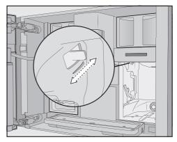
Push the slide control exactly 1 setting forward (for finer grinding) or one setting backward (for coarser grinding).
