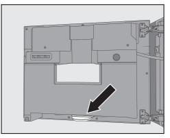
The drip tray is located at the bottom on the inside of the appliance door.
