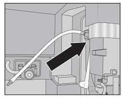
Connect together the angular molded hose and longer milk pipework. Start by attaching the top of the molded hose to the central spout. The black connecting piece should be pointing to the rear.
