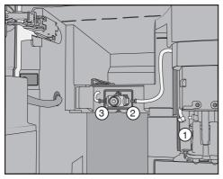
Detach the milk pipework from the dispensing unit on the central spout ① and from the milk valve silicone seal (② and ③).
