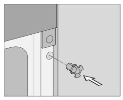
■ Insert the mounting aid into the hole in the front frame.
