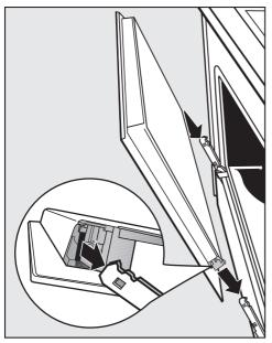
Hold the door securely on both sides and carefully install it back into the hinge retainers.
