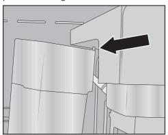
Attach the milk valve cover as follows: insert the pin in the top righthand corner and swivel the cover backward until a proper fit is achieved.
