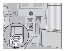
■ Pull the cleaning cartridge holder forward to remove it.
