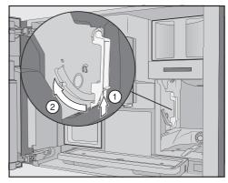
■ Press the button under the handle of the brew unit ① and, while doing so, turn the handle forward ②.
