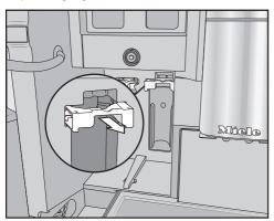
Pull the descaling cartridge holder forward.
