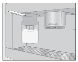
Push the milk flask back into the coffee machine until it clicks into place.
