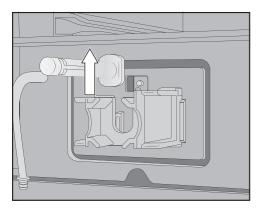
Pull the stainless steel bolt upward and out.
