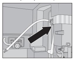
Connect together the angular molded hose and longer milk pipework. Start by attaching the top of the molded hose to the central spout. The black connecting piece should be pointing to the rear.
