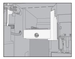
Remove the milk valve cover. Press on the recessed grip to unlock the cover.
