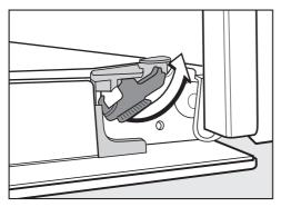
Release the locking clamps by turning them as far as they will go. You could damage the oven if you remove the door incorrectly.
