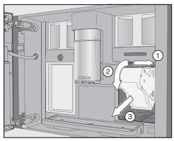
Pull the brew unit to the side 1 first and then pull out to the front 3. Tilt the brew unit forward 2.
