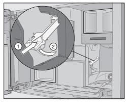
Press the button under the handle of the brew unit ① and, while doing so, turn the handle backward ②. **Tip:** If you are unable to turn the brew unit handle, apply firm pressure to the sides of the brew unit.
