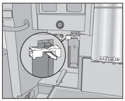
Pull the descaling cartridge holder forward.
