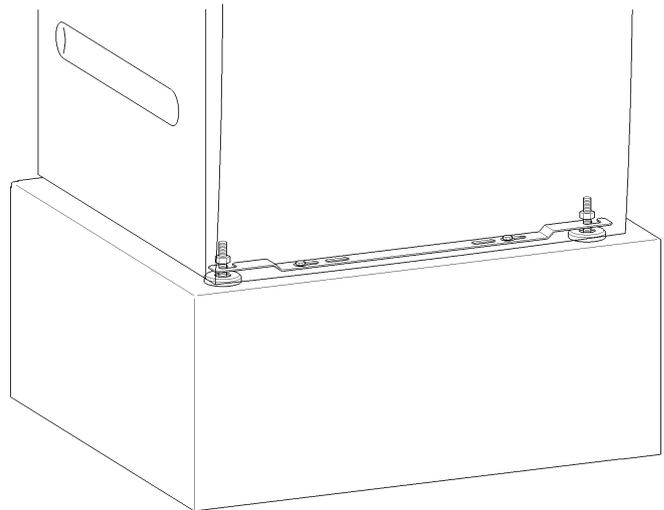
The anchors provided can be used to bolt the machine to the floor by both front feet. The fasteners provided are intended for use in bolting the machine to a concrete floor.
