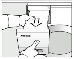
Remove the condensed water container.
