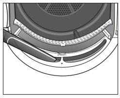
Use a vacuum cleaner with a long crevice nozzle attached to remove any visible lint from the upper air flow openings.
