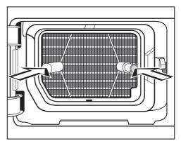
Push the plinth filter in completely.
