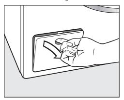
Open the drain pump flap.
