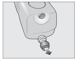
Remove the cover cap from the UltraPhase 1 detergent cartridge included with the delivery.
