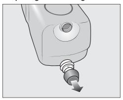
Remove the cover cap from the cartridge.
