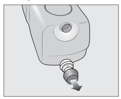
Remove the cover cap from the UltraPhase 2 detergent cartridge included with the delivery.
