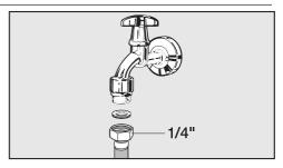
■ Screw the supplied brass compression fitting, with the 3/4" BPT end, tightly onto the water connector of the coffee machine. (Tighten the compression fitting by hand, do not use a tool.) The fitting includes an opening for standard 1/4" piping.
