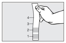
■ Dip the test strip in your drinking water for approximately one second, then shake off any excess water. The result will be evident after about a minute.
