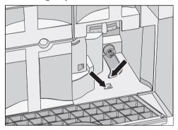
Carefully clean and dry the surface that the water container sits on, particularly the slots.
