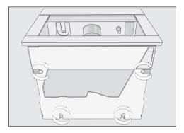
Unscrew the four feet on the underside of the unit by about 1/16"
