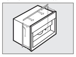
■ If there is no sealing strip around the installation recess, stick the Miele sealing strip onto the appliance from behind before putting it into the recess.
