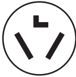
3-wire receptacle (10-30R)
