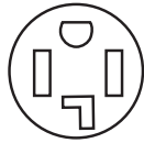
4-wire receptacle (14-30R)
