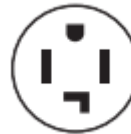
4-wire receptacle (14-30R)
