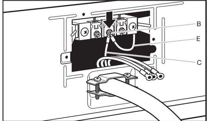
Connect neutral ground wire (E) and neutral wire (white or center) (C) of power supply cord under center terminal block screw (B). Tighten screw.
