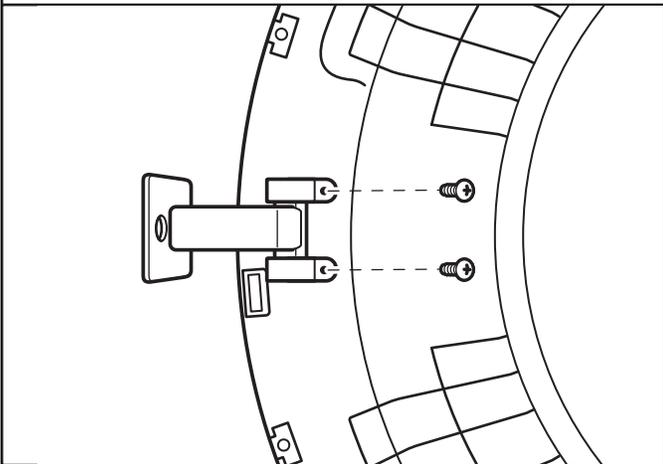
Lift off inner door assembly. Using a Phillips screwdriver, remove the two screws securing the rotating assembly to the door.
