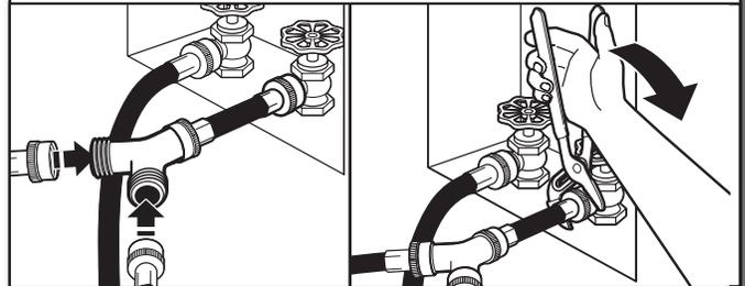
Attach one of the 5 ft. (1.5 m) inlet hose ends to the “Y” connector. Attach washer cold inlet hose to other side of “Y” connector. Screw on coupling by hand until it is seated on connector. Using pliers, tighten the couplings an additional 2/3 turn.
