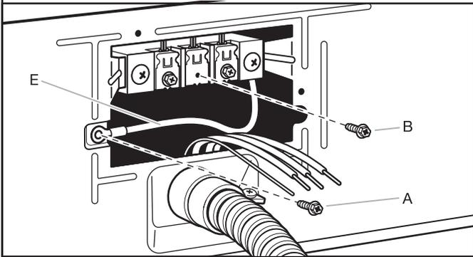
Remove center terminal block screw (B). Remove neutral ground wire (E) from green external ground conductor screw (A).
