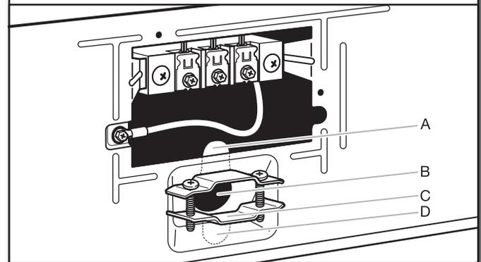
Remove the screws from a 3/4" (19 mm) UL Listed strain relief. Put the tabs of the two clamp sections (C) into the hole below the terminal block opening (B) so that one tab is pointing up (A) and the other is pointing down (D), and hold in place. Tighten strain relief screws just enough to hold the two clamp sections (C) together.
