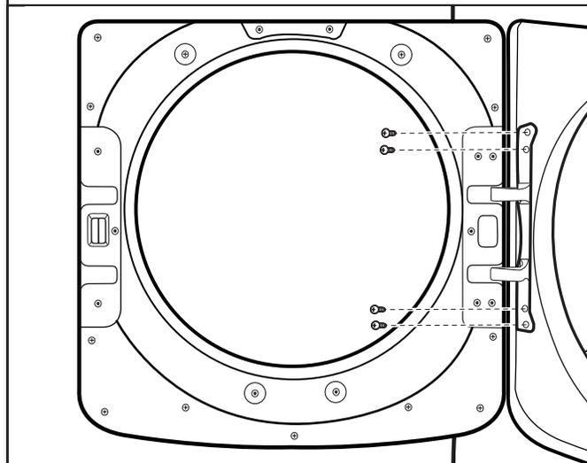
Using a T25® screwdriver, reinstall the four screws securing the door hinge to the dryer.
