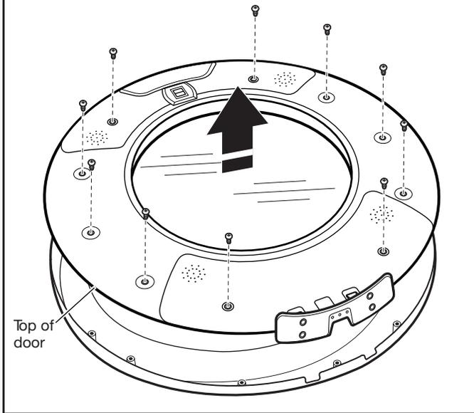
Position the door with the inside of the door facing up. Using a Phillips screwdriver, remove the 10 screws securing the inner door to the outer door.
