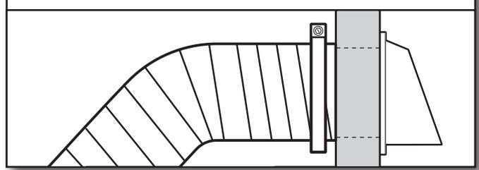
Vent must fit over the exhaust hood. Secure vent to exhaust hood with 4" (102 mm) clamp. Run vent to dryer location using straightest path possible. Avoid 90° turns. Use clamps to seal all joints. Do not use duct tape, screws, or other fastening devices that extend into interior of vent to secure vent, because they can catch lint.
