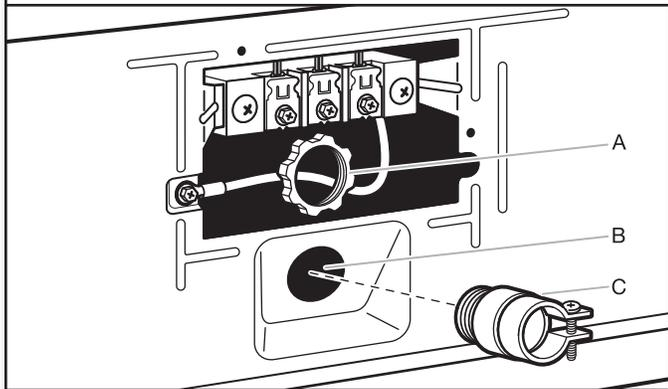
Unscrew the removable conduit connector (A) and any screws from a 3/4" (19 mm) UL Listed strain relief. Put the threaded section of the strain relief (C) through the hole below the terminal block opening (B). Reaching inside the terminal block opening, screw the removable conduit connector (A) onto the strain relief threads and tighten securely.
