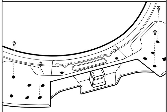
Using a T25® screwdriver, reinstall the latch plate on the opposite side from which it was removed with the four screws removed earlier.
