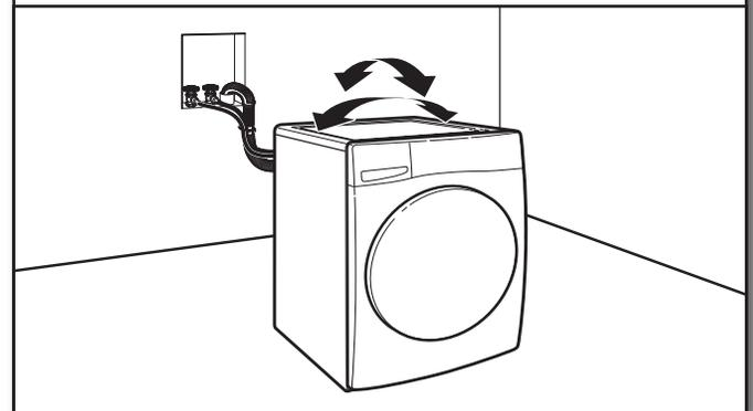
Grip washer from top and rock back and forth, making sure all four feet are firmly on floor. Repeat, rocking washer from side to side. If washer rocks, go to step 15 and adjust leveling feet. If all four feet are in firm contact with floor, go to Step 16.
