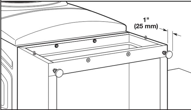
The pedestal arrives with the feet tight against the bottom of the unit. Using a 1/4" hex-head ratchet or open-end wrench, lower the feet approximately 1" (25 mm) away from the bottom of the pedestal.
