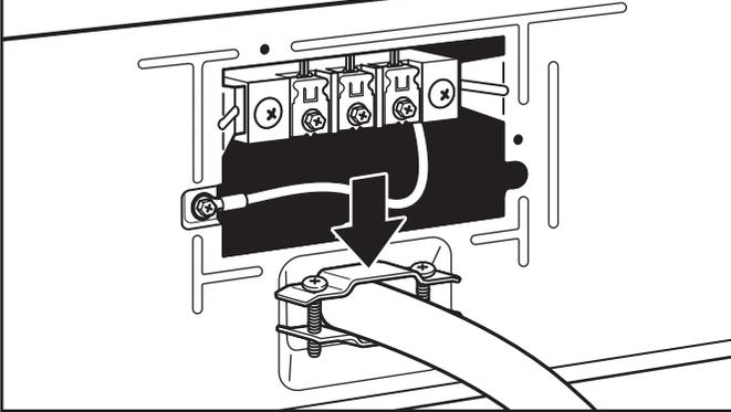
Put power supply cord through the strain relief. Be sure that the wire insulation on the power supply cord is inside the strain relief. The strain relief should have a tight fit with the dryer cabinet and be in a horizontal position. Do not further tighten strain relief screws at this point.
