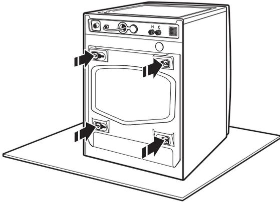
Locate the transport bolts on rear of washer. Transport bolts must remain in washer while pedestal is installed. When laying the washer on its back, hold the base down on the floor. Do not remove the plastic film, corner posts, or top cap.
