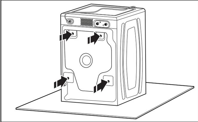
Locate four transport bolts on rear of washer.
