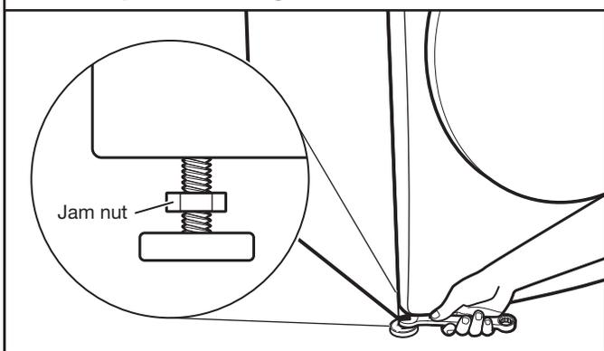
If washer is not level, use a 9/16" (14 mm) open-end or adjustable wrench to turn jam nuts clockwise on feet until they are about 1/2" (13 mm) from the washer cabinet. Then turn the leveling foot clockwise to lower the washer or counterclockwise to raise the washer. Do not exceed 2" (50 mm) from bottom of foot to bottom of cabinet. Recheck levelness of washer and that all four feet are firmly in contact with the floor. Repeat as needed.
