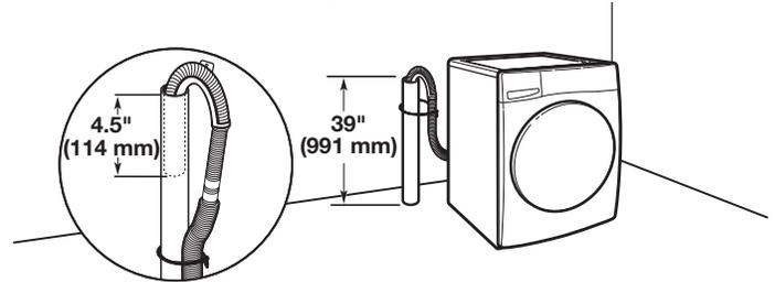
Minimum diameter for a standpipe drain: 2" (51 mm). Minimum carry-away capacity: 17 gallon (64 L) per minute. A 1/4" (6 mm) diameter to 1" (25 mm) diameter Standpipe Adapter Kit is available (Part Number 3363920). Top of standpipe must be at least 39" (991 mm) from the floor; install no higher than 96" (2.44 m) from bottom of washer. If you have an overhead sewer and need to pump higher than 96" (2.44 m), a sump pump and associated hardware are needed. See "Alternate parts."
