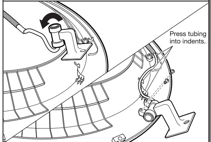
Rotate bottom of assembly 180° towards you and secure assembly with the two screws removed earlier, using a Phillips screwdriver. Press tubing into indents.
