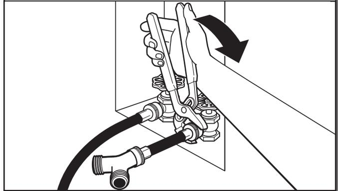
Using pliers, tighten the couplings with additional 2/3 turn. **NOTE:** Do not overtighten. Damage to the coupling can result.
