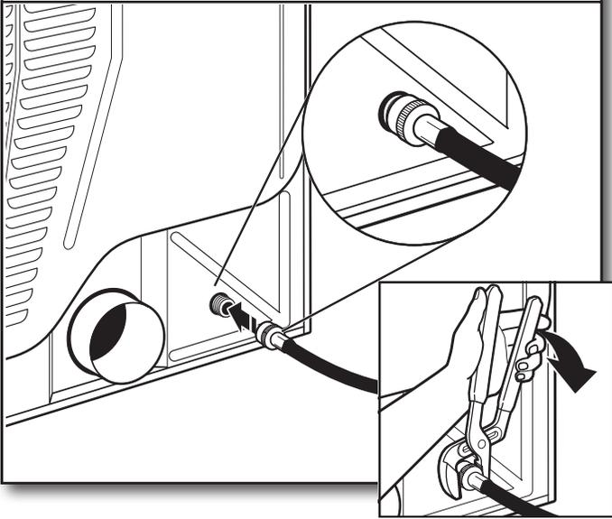
Remove protective cap from water inlet valve. Attach other end of long hose to fill valve at bottom of dryer back panel. Screw on coupling by hand until it is seated on fill valve connector. Using pliers, tighten the couplings an additional 2/3 turn.
