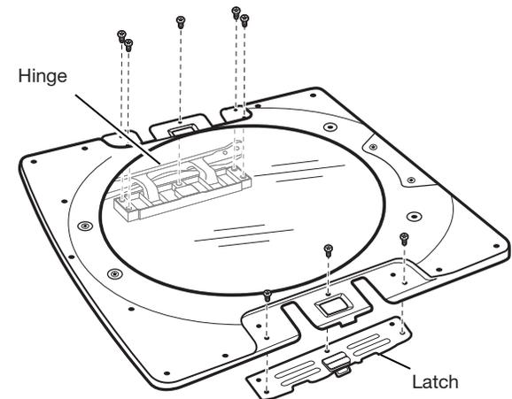
Using a T25® screwdriver, remove the three screws securing the latch plate and the five screws holding the hinge assembly in place.
