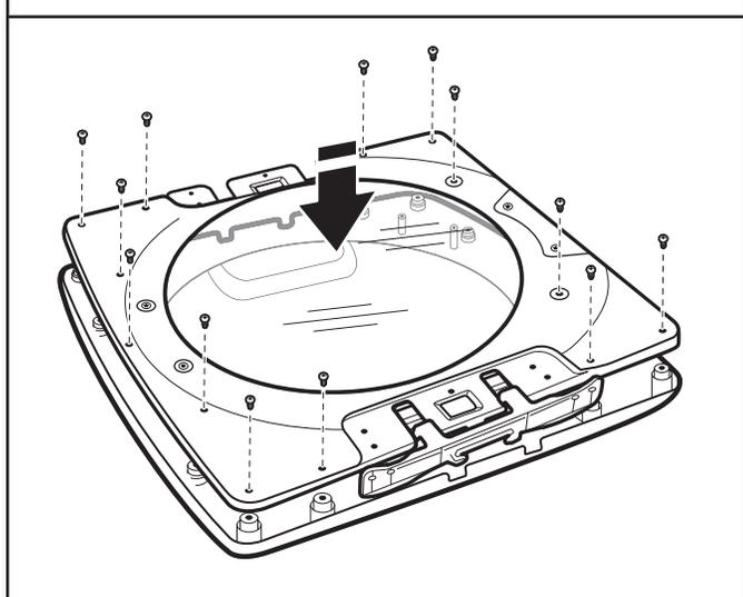
Position the inner door on the outer door assembly. Using a Phillips screwdriver, secure with the 13 screws removed earlier.
