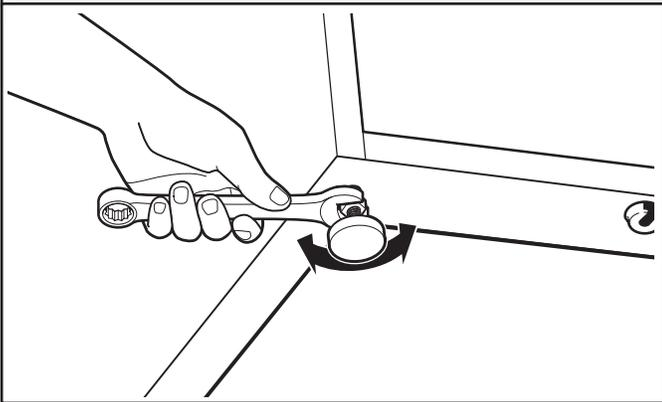
When the washer/dryer is level, use a 9/16" open-end wrench to securely tighten all four jam nuts against the pedestal.
