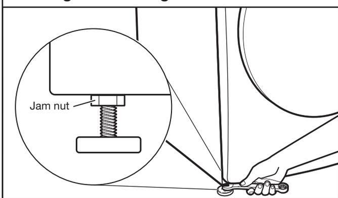
When washer is level and all four feet are firmly in contact with the floor, use a 9/16" (14 mm) open-end or adjustable wrench to turn jam nuts counterclockwise on leveling feet tightly against washer cabinet.
