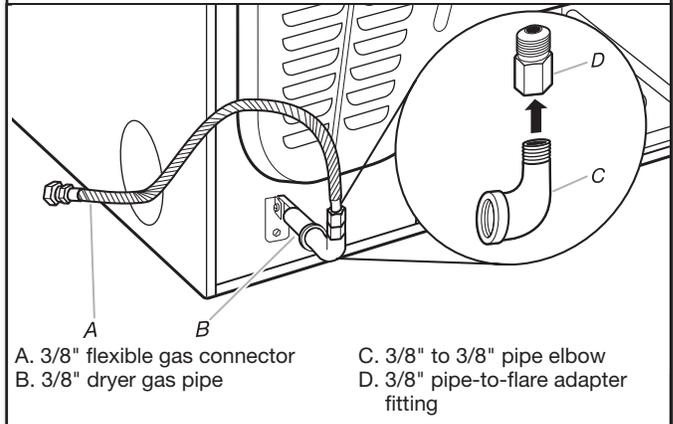
A combination of pipe fittings must be used to connect dryer to existing gas line. A recommended connection is shown. Your connection may be different, according to supply line type, size, and location.
