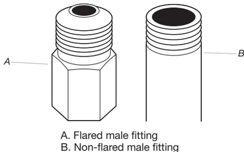
Remove red cap from gas pipe. Using a wrench to tighten, connect gas supply to dryer. Use pipe-joint compound on threads of all non-flared male fittings. If flexible metal tubing is used, be sure there are no kinks.
