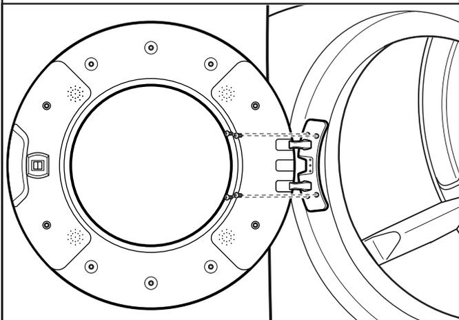
**Doors with electrical wiring:** Pull the wire through the front panel opening before reinstalling the door.
