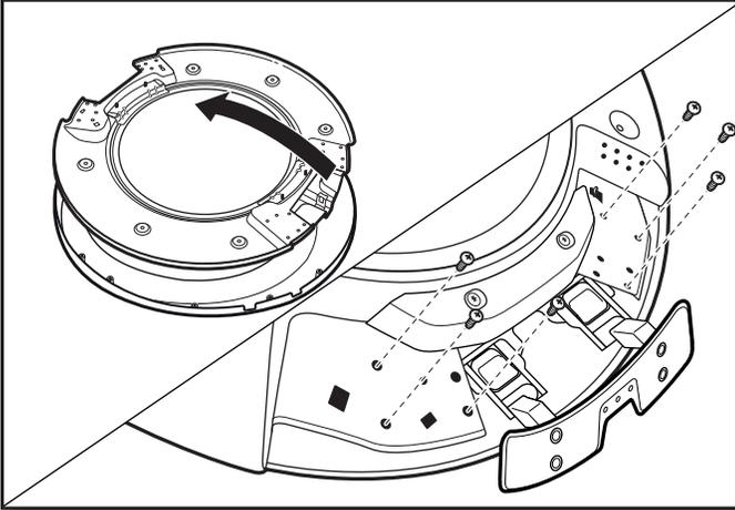
Flip over the inner door to the left. Using a T20® screwdriver, reinstall the hinge assembly on the opposite side from which it was removed.
