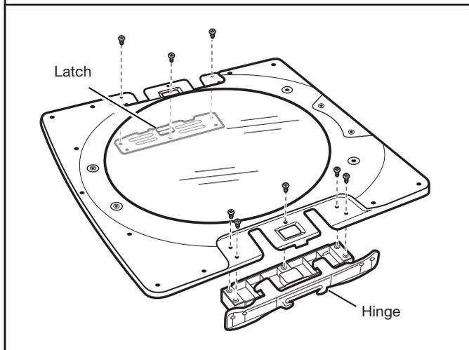
Using a T25® screwdriver, reinstall the latch plate and hinge assembly on the opposite sides from which they were removed.
