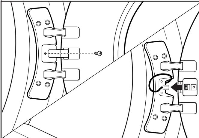
Using a Phillips screwdriver, remove middle screw in hinge. Disconnect wiring. Tuck wiring into opening.
