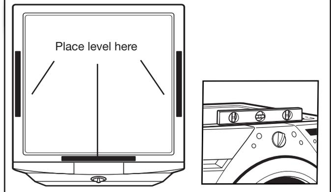
Place a level on top edges of washer/dryer, checking each side and front. Rock washer/dryer back and forth to make sure all four feet make solid contact with floor.
