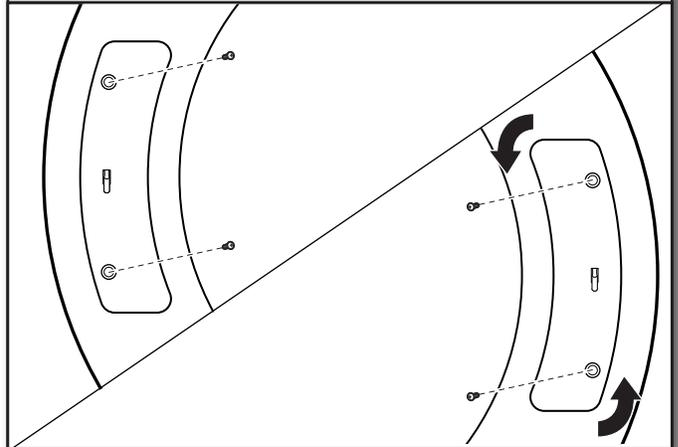
Using a T25® screwdriver, remove the two screws securing the door strike to the door frame of the dryer. Rotate the strike 180° and attach to the opposite side of dryer door frame with the two screws removed earlier, as shown.
