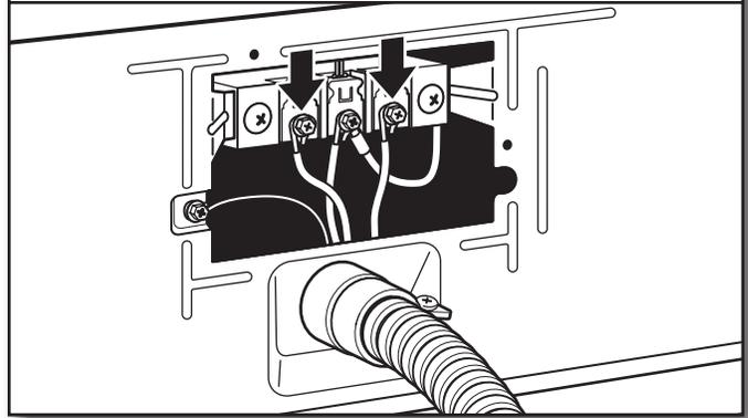
Place hooked ends of remaining direct wire cable wires under outer terminal block screws (hooks facing right). Squeeze hooked ends together and tighten screws. Finally, reinsert tab of terminal block cover into slot of dryer rear panel. Secure cover with hold-down screw. Now go to "Venting Requirements."
