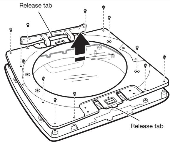
Position the door with the inside of the door facing up. Using a Phillips screwdriver, remove the 13 screws securing the inner door to the outer door. Lift off the inner door and set aside.
