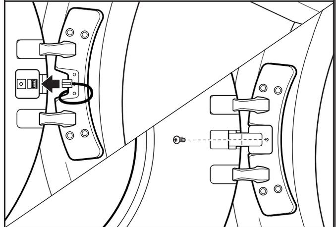
Plug in wire. Using a Phillips screwdriver, secure the rotating assembly to the hinge with the screw removed earlier.
