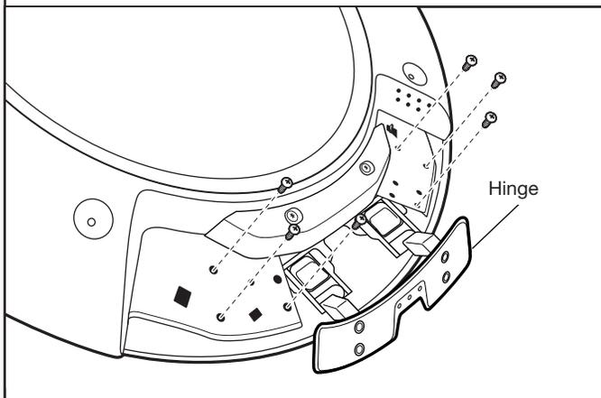
Using a T20® screwdriver, remove the six screws holding the hinge assembly in place.
