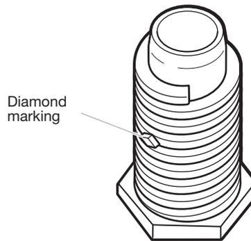
Examine leveling legs and locate the diamond marking. Screw legs into leg holes by hand – use a wrench to finish turning legs until diamond marking is no longer visible.
