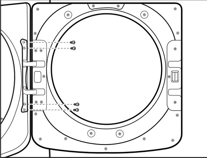
Using a T25® screwdriver, remove the four screws securing the door hinge to the dryer and lift up and out to remove the door. Place the door on a soft towel or other non-scratch surface. Retain or set aside the four screws.
