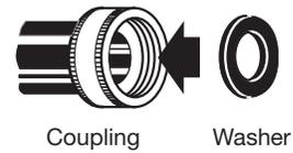
**IMPORTANT:** To avoid leaks, check that your water inlet hoses have flat washers at both ends. Washer must be connected to water faucets with new inlet hoses with flat washers (not provided). Do not use old hoses. Do not use hoses without washers.
