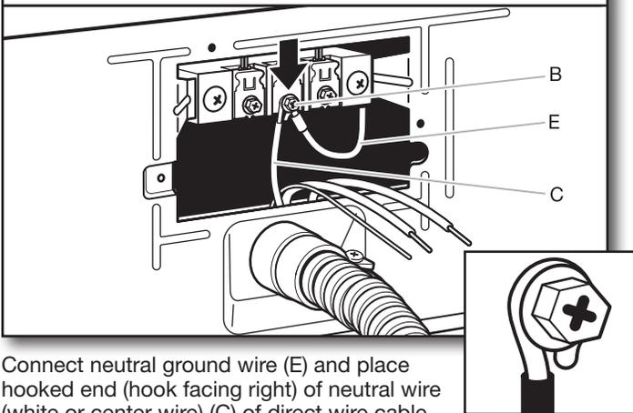
Connect neutral ground wire (E) and place hooked end (hook facing right) of neutral wire (white or center wire) (C) of direct wire cable under center screw of terminal block (B). Squeeze hooked ends together and tighten screw.
