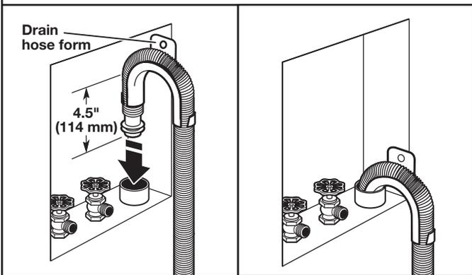
Place hose into standpipe (shown in picture) or over side of laundry tub.
