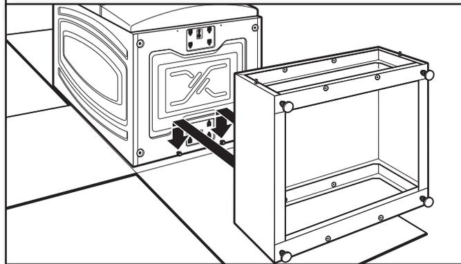
Move the pedestal against the washer/dryer bottom. Slide the pedestal's keyhole slots over the lower two partially installed screws.
