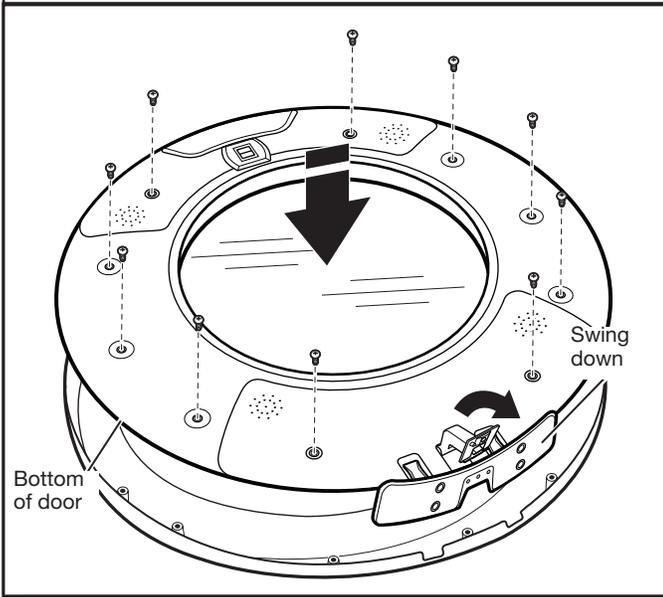
Position the door with the inside of the door facing up. Using a Phillips screwdriver, reinstall the 10 screws removed earlier, securing the inner door to the outer door.
