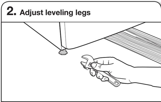
If dryer is not level, prop up using a wood block, use wrench to adjust legs up or down, and check again for levelness. Once dryer is level, make sure all four legs are snug against the floor and the dryer does not rock.
