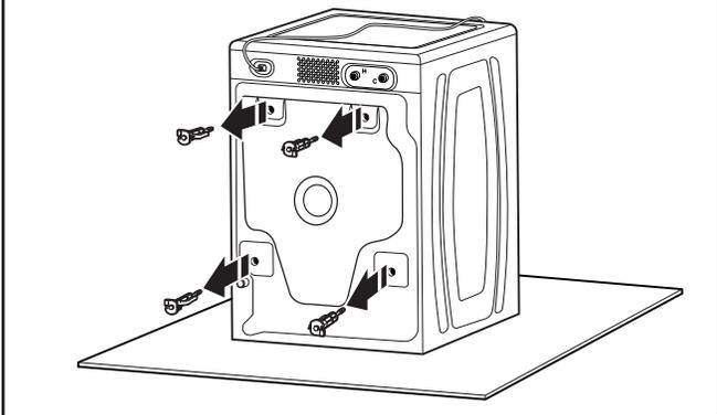
Loosen bolts with a 5/8" (16 mm) wrench. Slide each bolt and spacer to center of hole. Pull bolts and plastic spacers from back of washer. Discard bolts and spacers.
