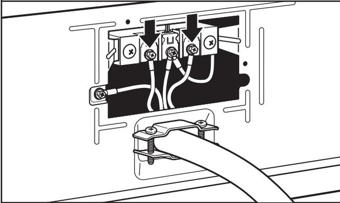
Connect remaining wires under outer terminal block screws. Tighten screws. Finally, reinsert tab of terminal block cover into slot of dryer rear panel. Secure cover with hold-down screw. Now go to "Venting Requirements."
