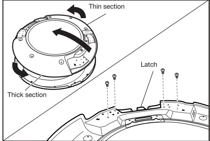
Flip and rotate the inner door 180° so that the thin section is at the top and the thick section is at the bottom. Using a T25® screwdriver, remove the four screws securing the latch plate in place.
