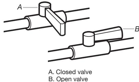
Open shut-off valve in supply line; valve is open when handle is parallel to gas pipe. Then, test all connections by brushing on an approved noncorrosive leak-detection solution. Bubbles will show a leak. Correct any leak found.
