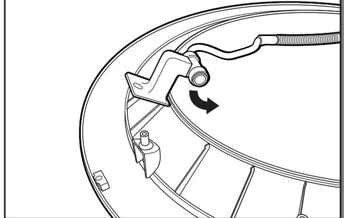
Reposition rotating assembly and tubing 180° to opposite side of the door.
