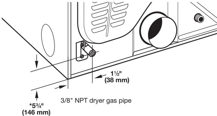
**\*NOTE:** If the dryer is mounted on a pedestal, the gas pipe height must be an additional 10" (254 mm) or 15.5" (394 mm) from the floor, depending on the pedestal model. For a garage installation, the gas pipe height must be an additional 18" (460 mm) from the floor.
