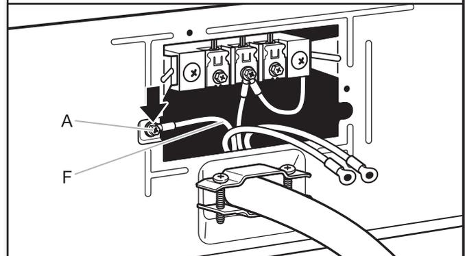
Connect ground wire (F) (green or bare) of power supply cord under green external ground conductor screw (A). Tighten screw.
