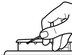
4. Replace the burner cap, making sure the alignment pins are properly aligned with the burner cap.
