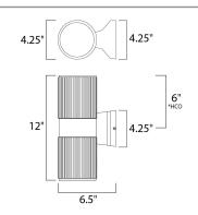
\*height from center of outlet to the top of the fixture  $% \left( t\right) =\left( t\right) \left( t$
