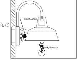
Step.3 Put the connected line into the electric box and fasten the light body with the decorative nut.
