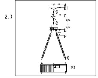
Step. 2: Attach appropriate amount of chain to loop to achieve desired mounting height. Thread wire through every 3rd loop of chain.
