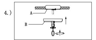
Step. 4: Pull canopy through screw ring up chian to ceiling to and tinghten sccurely.
