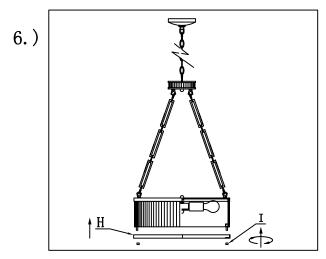
Step. 6: Install the bottom ring (H) on the body and lock screw(I).
