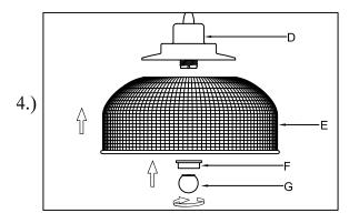
Step 4: Insert glass (E) into cup (D) and secure using Aluminum loop (F) provided , At last Screw (G) to the lamp holder.
