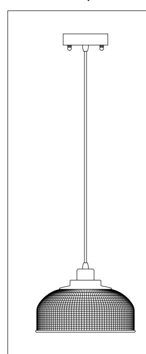
The fixture is designed to dim with a standard Triac forward phase dimmer. Dimming levels will vary by dimmer.
