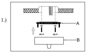
Step 1: Remove mounting bracket (A) from canopy (B) and install to electrical box.
