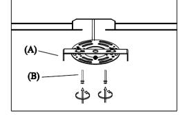
Step.1: 1: Remove mounting bracket (A) from fixture and install to electrical box using screws (B).
