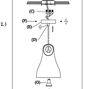
Step.2: Adjust wire length to desired mounting height, and tighten strain relief screws (D) to secure. Wire fixture to wires in outlet box. Green wire is for Ground. Install fixture to bracket and tighten screws (F) at the ends of the canopy (D) to secure. Install LED GU10 bulb (G).
