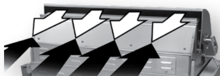
Be sure wind doesn't blow into the hood gap.
