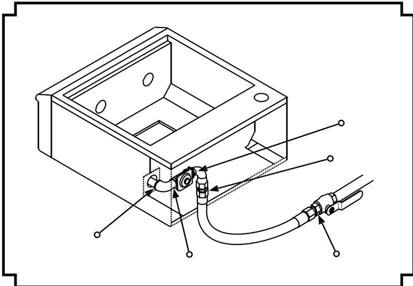
Figure 11-1 - Leak testing points when using natural gas.
