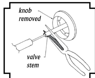
**Figure 14-2 - Adjusting brass burner low heat setting.**
