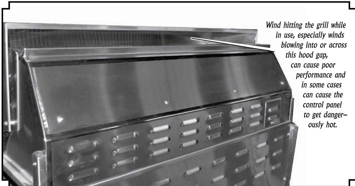
*Wind hitting the grill while in use, especially winds blowing into or across this hood gap, can cause poor performance and in some cases can cause the control panel to get dangerously hot.*
