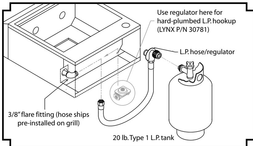
Figure 9-1 - Typical attachment to L.P. tank.
