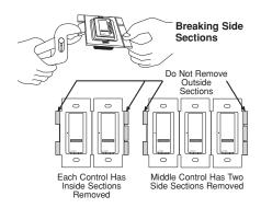
Reduction of the *Spacer System* switch load capacity *is required* when removing side sections. See table below.
