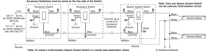
the wiring diagram but without Accessory Switches, and cap off the blue wire.
