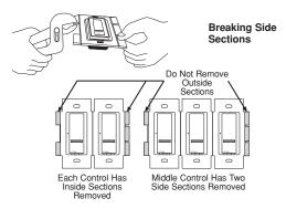
Reduction of the *Spacer System* Switch load capacity *is required* when removing side sections. See table below. The Accessory Switch does not require derating.
