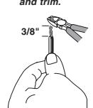
When making wire connections, twist and trim wires to the proper length as indicated:
