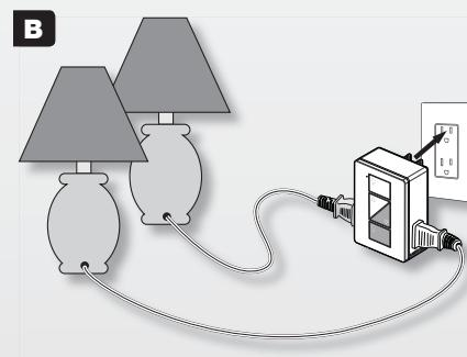
Insert the plug of the Plug-In Dimmer into the wall outlet
