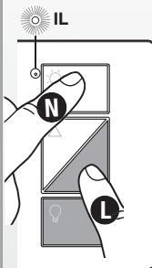
Press and hold **L** & **R** for 6 seconds until the indicator light (IL) flashes.
