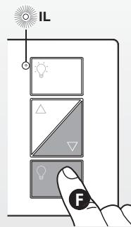
Press and hold **F** for 6 seconds until the indicator light (IL) flashes.
