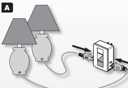
Turn the lamp on and plug the lamp cord into either Plug-In Dimmer receptacle.
